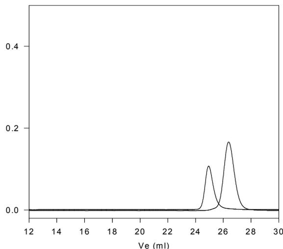
Size exclusion chromatography of polystyrene-*b*-polyisoprene<sub>1,4</sub> addition
