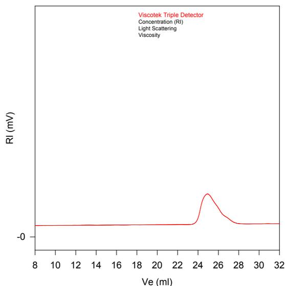
Size Exclusion Chromatography of poly(ethylene glycol)methyl ether: Poly (ethylene Oxide);
