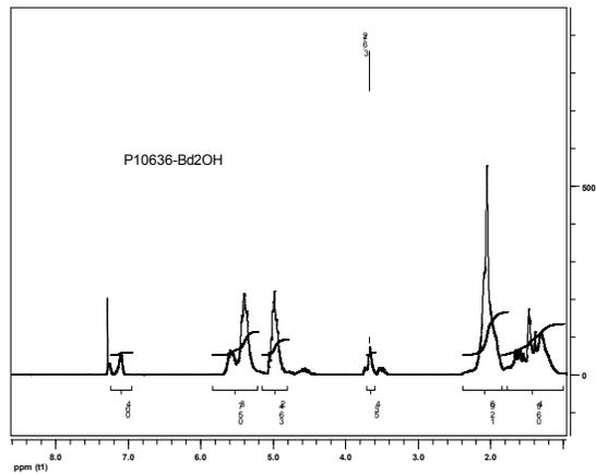
**<sup>1</sup>H NMR of the  $\alpha$ - $\omega$  Benzyl Chloride acid terminated Polybutadiene**
