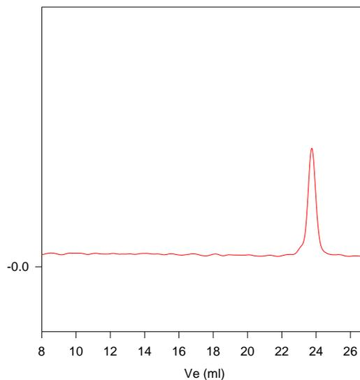
Size exclusion chromatograph of epoxy terminated poly(ethylene glycol) methyl ether:
