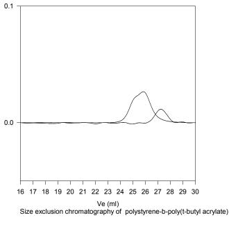
Polystyrene, M<sub>n</sub>=1500, M<sub>w</sub>=1800, PI=1.2
