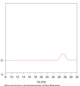
Size exclusion chromatograph of the Polymer; M<sub>a</sub>=2500, M<sub>w</sub>=2800 Mw/Mn =1.15
